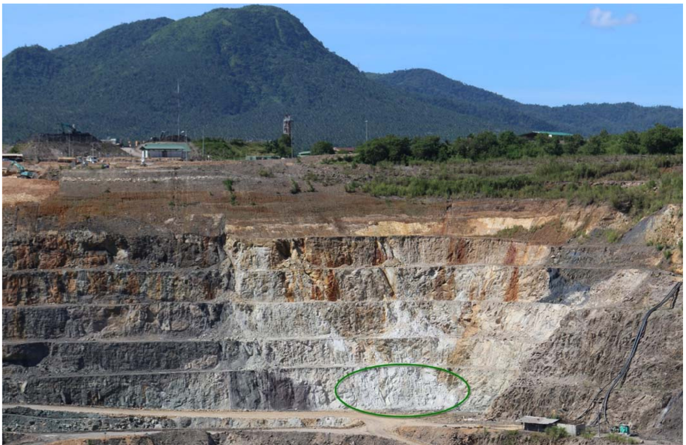
Figure 3: View of the Siana open pit Stage 4 West wall highlighting the estimated position of the planned U/G portal
