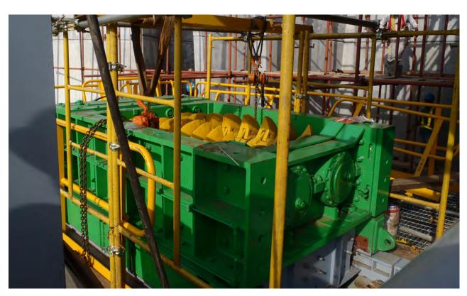
Primary rolls crusher, specifically chosen to handle wet ore.
