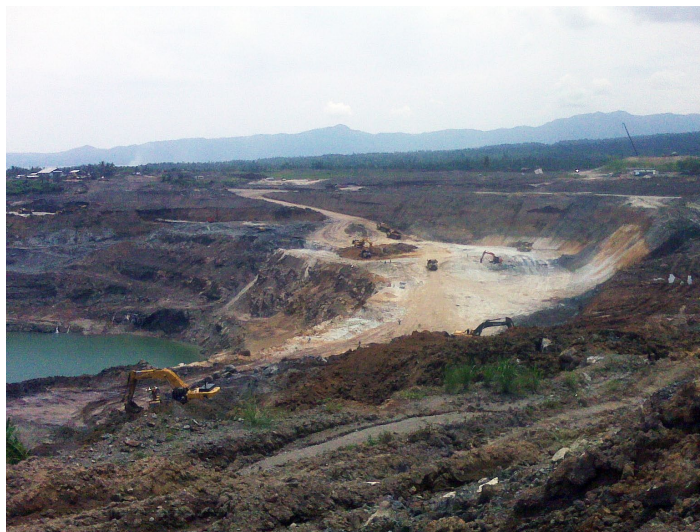
Open pit cut back activity and nearly dewatered pit.
