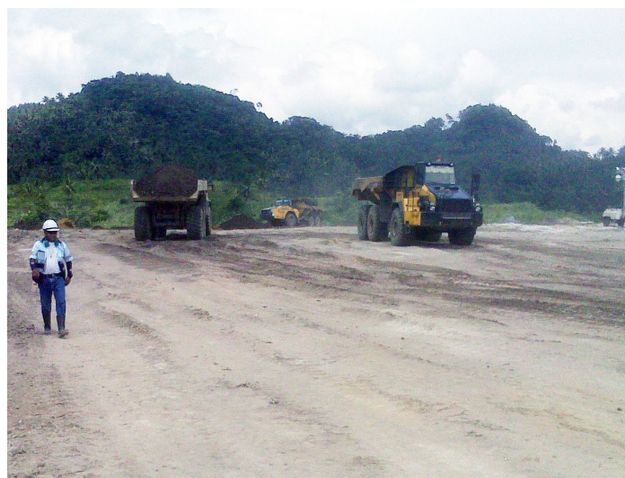
40 tonne six-wheel-drive articulated trucks cycling to the waste dump.
