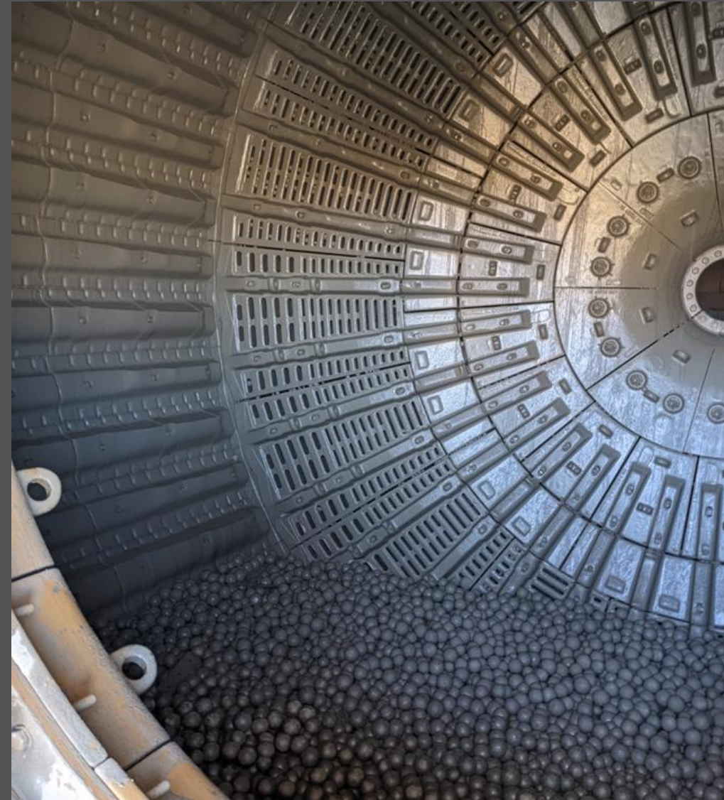
Mill discharge grates showing improved “pegging” in October
