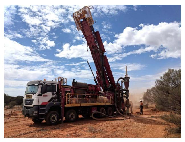
Figure 1: Reverse Circulation (RC) drill rig at the Centauri prospect, where drilling commenced in March 2019.
