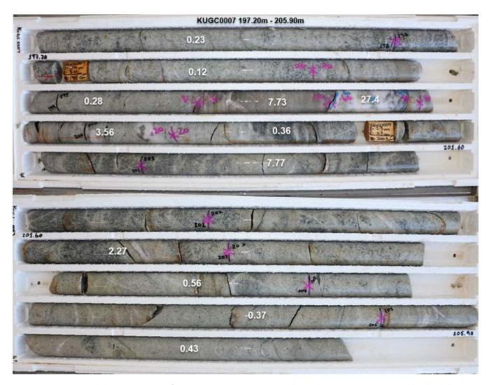
Figure 4: Diamond drill core – KUGC0007 from 197.2m to 205.9m. Veins, veinlets and micro-veins visible throughout the drill core.
