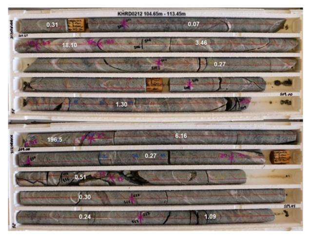
Diamond drill core – KHRD0212 from 104.65m to 113.45m. Veins, veinlets and micro-veins visible throughout the drill core.
