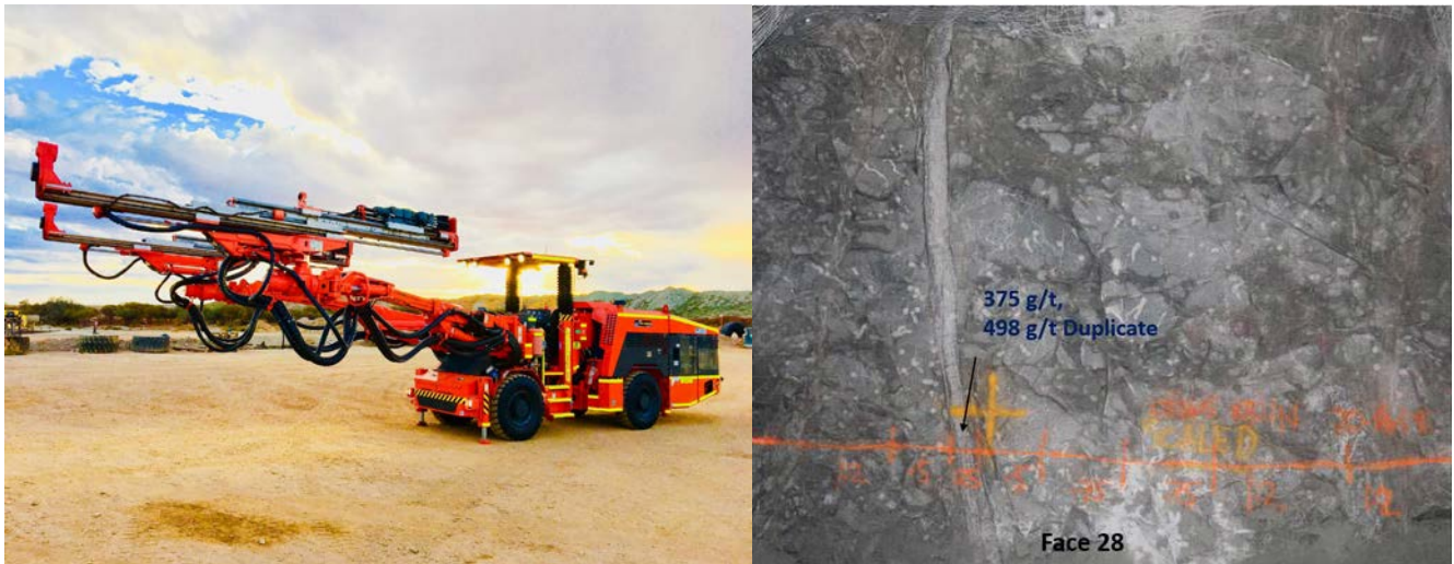
Figure 4: Delivery of Pit N Portals new DD321 Jumbo, allowing for tighter mining widths, optimising stoping with the narrow orebodies. Second image shows the Riverrun C5145 Development Face and ore zone grading at 498g/t at ~0.25m width.
