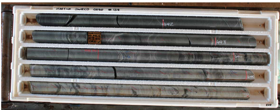
Figure 12: Photo showing hole SWDD0040 between 491-496 metres. High strain deformation and pervasive alteration persists down to 680m. This zone is indicative of strong shear and high fluid flow.
