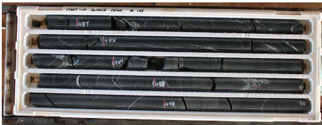
Figure 11: Photo showing hole SWDD0040 between 487-491 metres. High strain deformation and pervasive alteration persists down to 680m. This zone is indicative of strong shear and high fluid flow.
