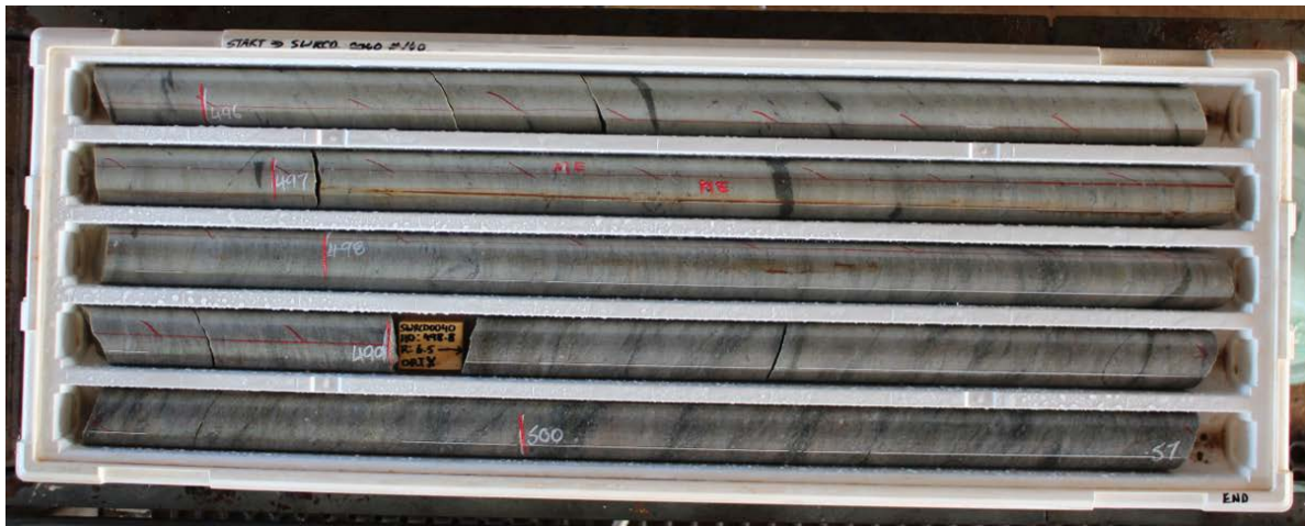
Figure 13: Photo showing hole SWDD00040 between 496-501 metres. High strain deformation and pervasive alteration persists down to 680m. This zone is indicative of strong shear and high fluid flow.
