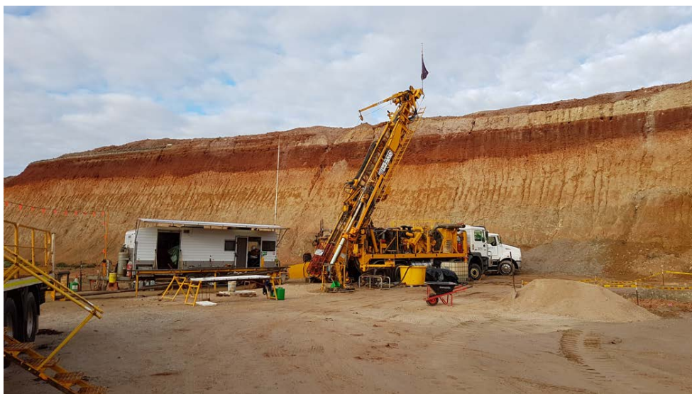
Figure 5: DDH1 drilling at KOTH for metallurgical heap leach samples.
