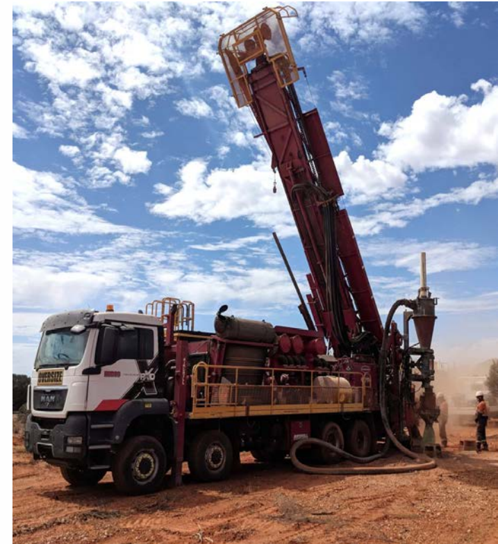
Near-mine regional exploration – RC drilling in progress
