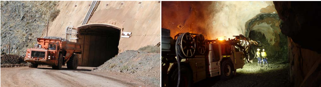
Figures 3 and 4: Underground portal entrance (left) and stope (right) (photographs supplied by Gold Fields Limited)
