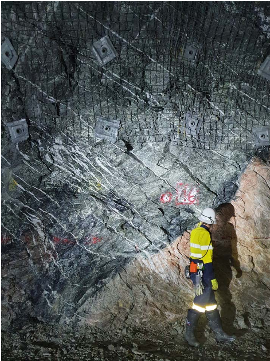
Figure 2. An underground mine geologist examining the intense veining along the ‘damage zone’, between the Granodiorite and Ultramafic contact.
