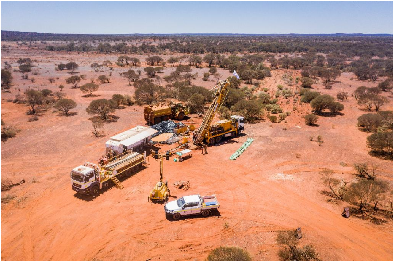
Figure 1. DDH1 drilling core at satellite pit area for geotechnical purposes.
