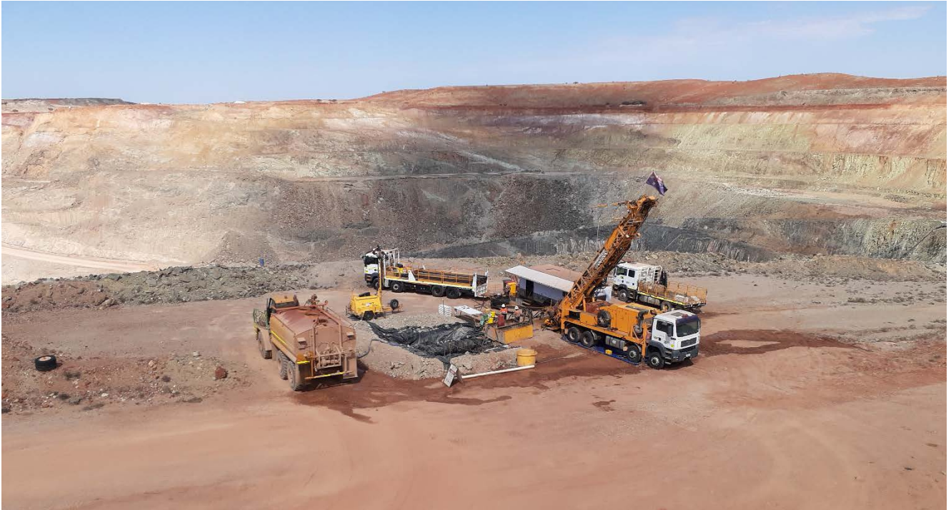
Figure 9: Drilling of 200m geotechnical diamond drill hole in the NE section of the open pit.
