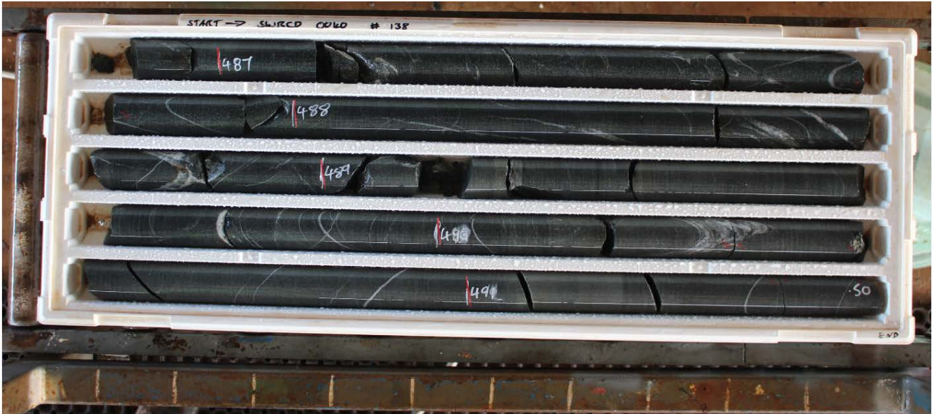
Figure 6: Photo showing hole SWDD00040 between 487-491 metres. High strain deformation and pervasive alteration persists down to 680m. This zone is indicative of strong shear and high fluid flow.
