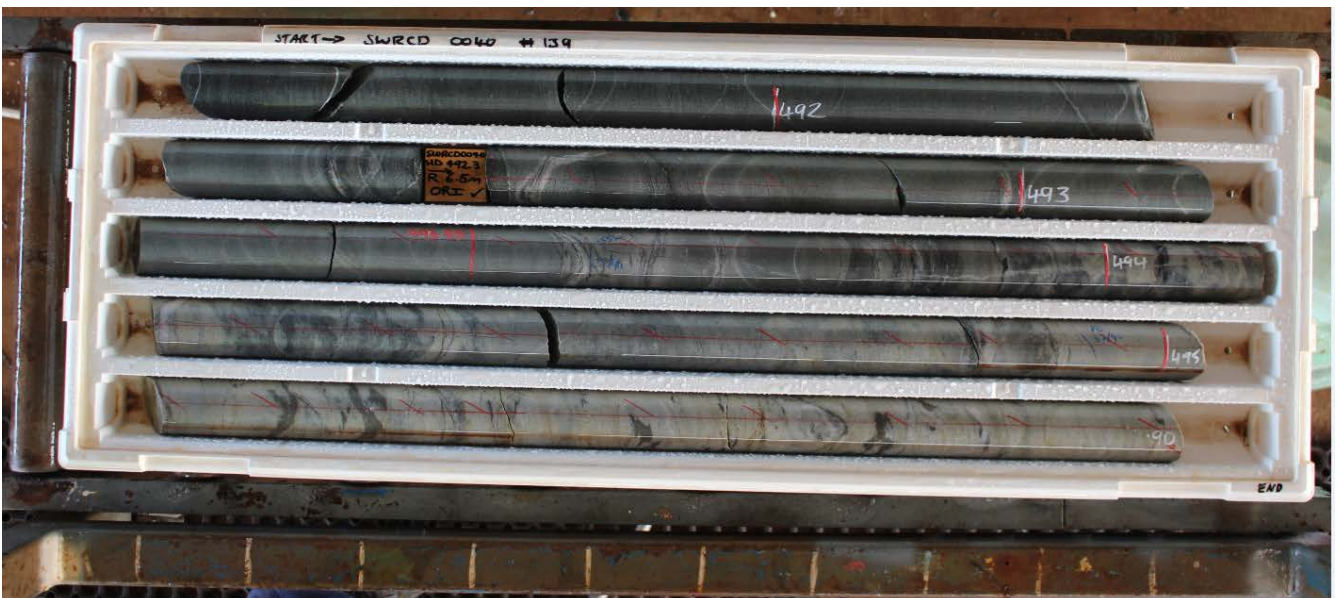
Figure 7: Photo showing hole SWDD00040 between 491-496 metres. High strain deformation and pervasive alteration persists down to 680m. This zone is indicative of strong shear and high fluid flow.
