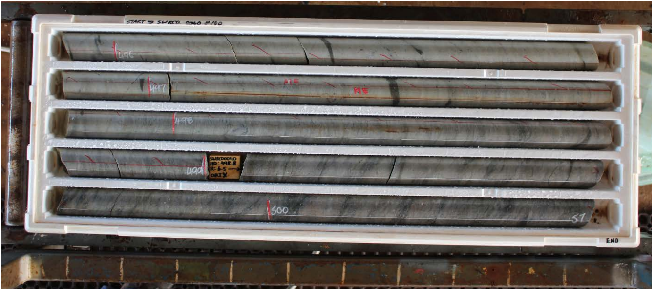
Figure 8: Photo showing hole SWDD00040 between 496-501 metres. High strain deformation and pervasive alteration persists down to 680m. This zone is indicative of strong shear and high fluid flow.
