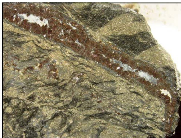
Siana zinc sulphide-gold vein in pyritic limestone -SMDD105
