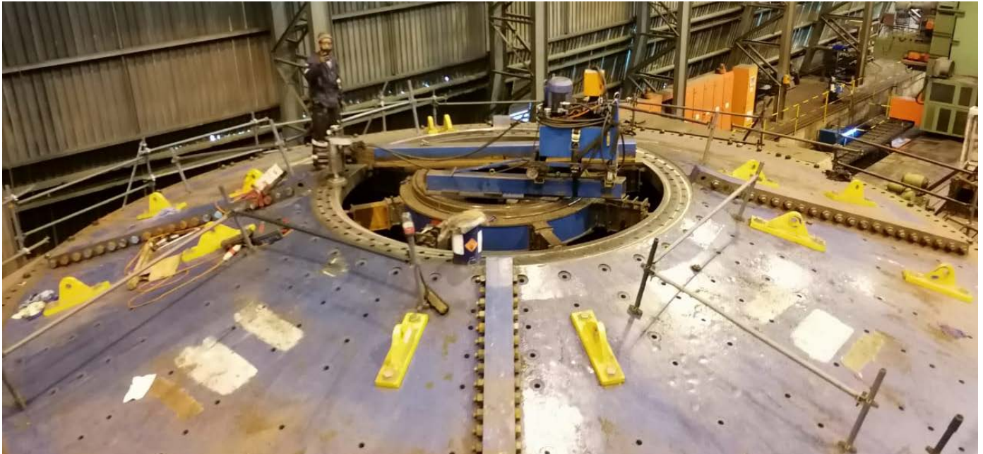
Figure 2: Mill feed end head during machining at a Johannesburg workshop.
