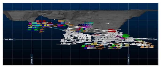
*Figure 6:* Projected Long Section view looking west of the King of the Hills Deposit, illustrating the current pit, the North Mine underground workings and the proposed mine design for both the North and Central mining areas.
