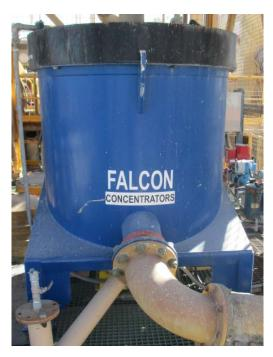
Figure 2: Falcon SB Gravity Concentrator.
