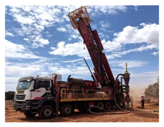
Figure 4: Reverse Circulation (RC) drill rig at the Centauri prospect, where drilling commenced in March 2019.
