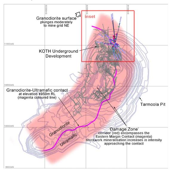
**Figure 1:** Schematic plan view of King of the Hills gold mine, showing current pit outline and underground development, and the recently reported drill-holes.
