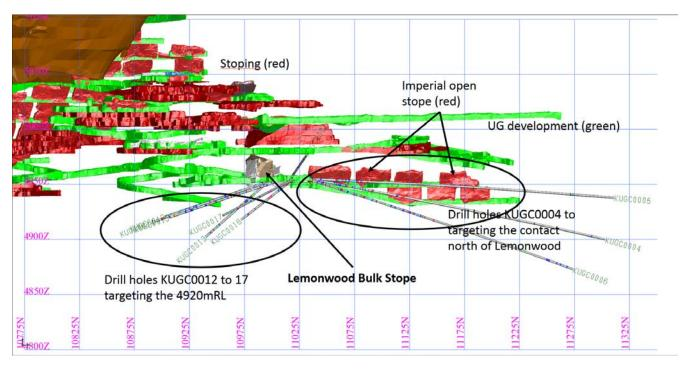
**Figure 3:** Long section view of the in-fill drill targeting the mineralisation in the Lemonwood bulk stope area located along the eastern contact for drill holes KUGC0001 to 6 and KUGC0012 to 17.
