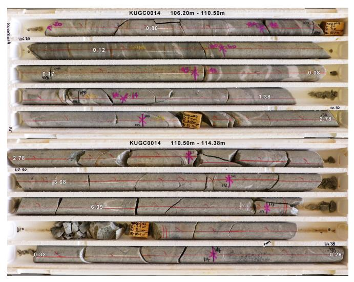
Figure 6: Photograph – Lemonwood Bulk Stope Area drill core (KUGC0014 106.2m–114.38m).
