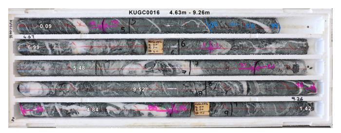
Figure 7: Photograph - Lemonwood Bulk Stope Area drill core (KUGC0016 4.63m-9.26m).
