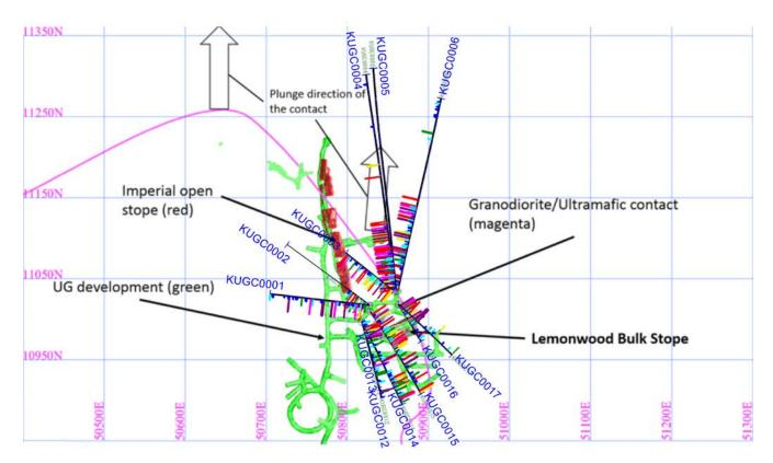
**Figure 2:** Plan view of the in-fill drill targeting the mineralisation in the Lemonwood bulk stope area located along the eastern contact for the drill holes KUGC0001 to 6 and KUGC0012 to 17.
