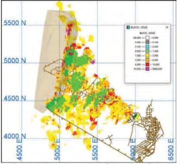
An oblique view looking north representing the Pedersen deposit (Darlot gold mine) is shown below, with current development (brown), stopes (green) and the block model at a 2 g/t cut-off.
