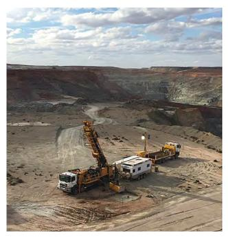
Figure 7: DDH1 drilling at KOTH for metallurgical heap leach samples.
